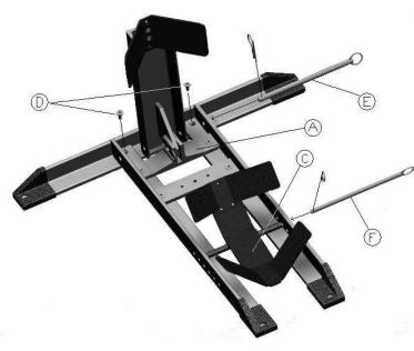
Step1: Using screws (D), attach the Base Bar (B) to the Main Unit (A). (3/16 allen wrench required, torque between 16 - 18 ft-lbs)
